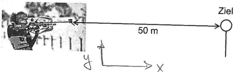
ln x:  $x = v_0 t \Rightarrow t = \frac{50 \text{ m}}{350 \frac{\text{m}}{\text{s}}} = 0,143 \text{ s}$
