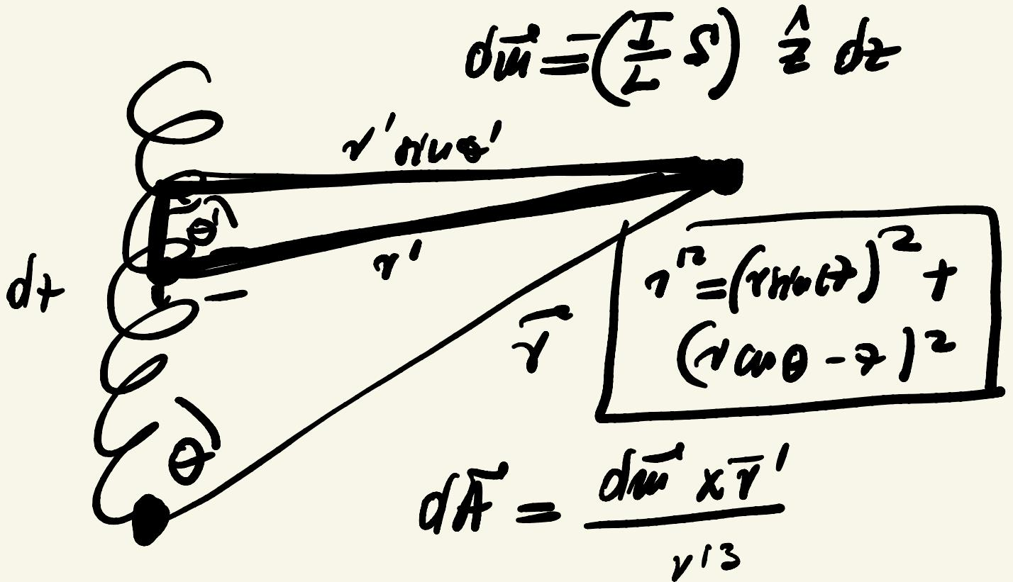
$$\vec{A} = - \underbrace{\left( \frac{I}{L} S \right)}_{\text{dimensions}} \int \frac{dz \hat{z} \times \vec{r}'}{r'^3}$$
