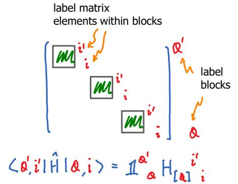
Separate diagonalization of each block yields simultaneous eigenbasis of  $\hat{H}$  and  $\hat{Q}$ .
